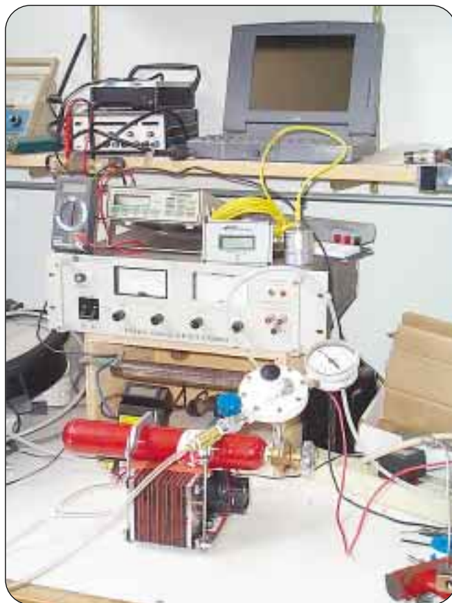
The homebrew fuel cell on the test bench.
